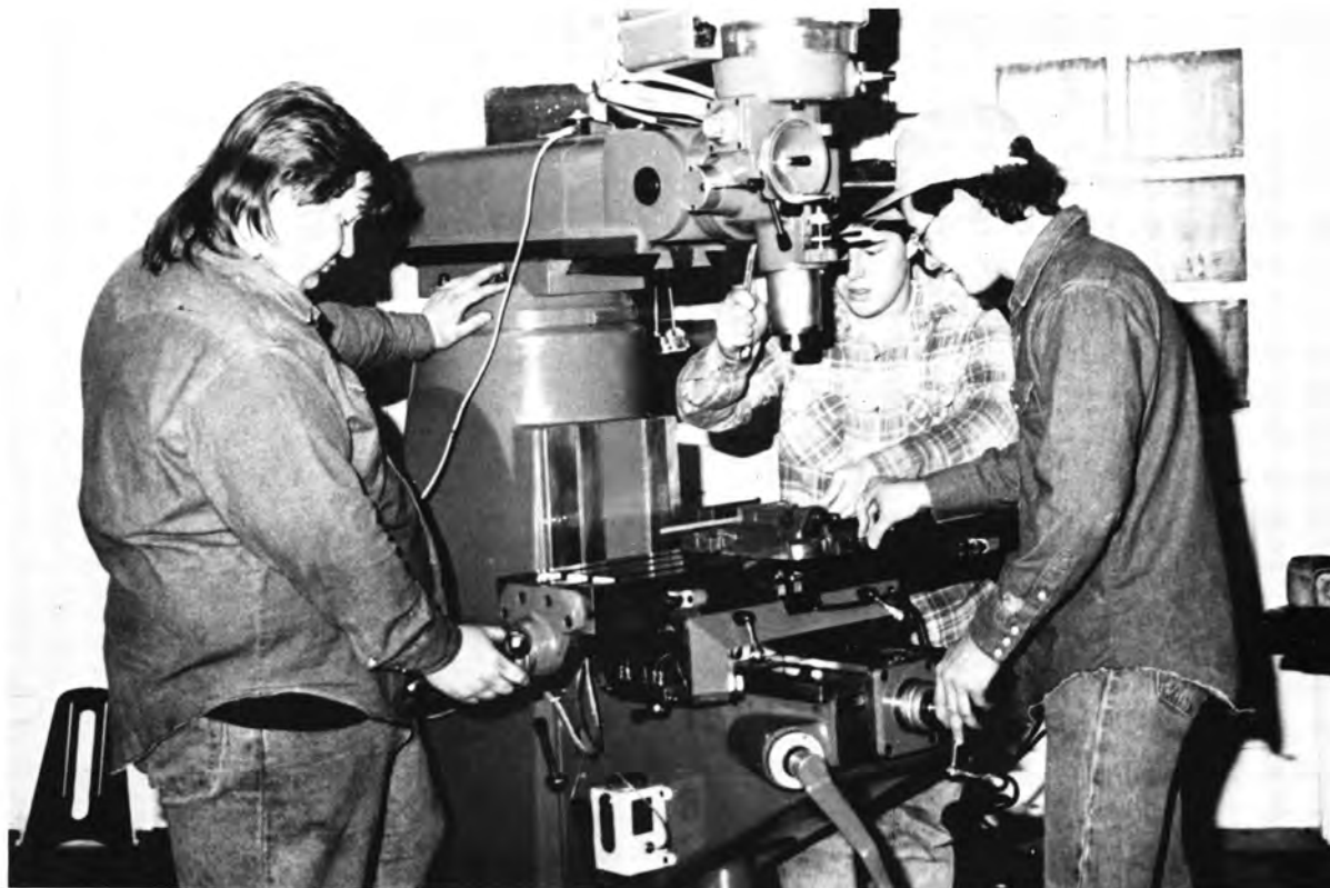
Sophomores Paul Neiberger, of Miami, Robbie Parrish, of Nowata, and Rusty Wilmoth, of Fairland, cut a pattern on a vertical milling machine in the college metal fabrication program.
